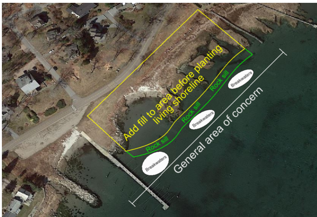
Figure 5: Potential design for a living shoreline and protective devices (Photo taken from Google earth, overlay created using Microstation)
